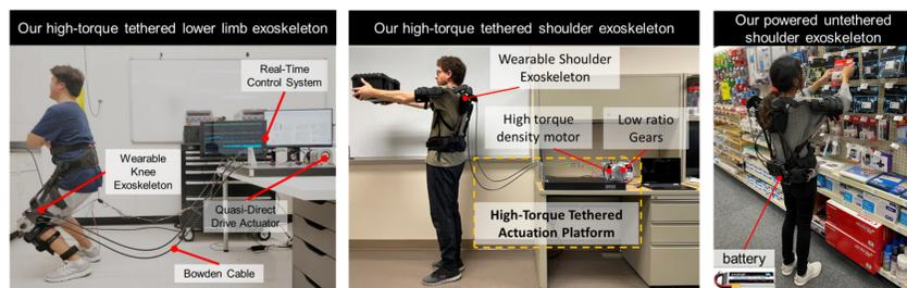
Figure 1. Evolution of exos design: transition from lab-based to real-life workplace oriented.
